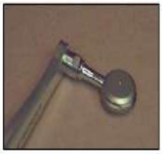
Figure 75. Pedal axie extender. This steel extender effectively lengthens the axie 20 mm.
