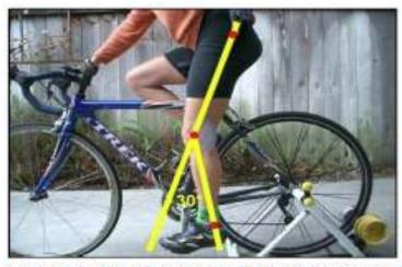
Figure 12. Seat height. A seat height that results in 30° of knee flexion is a good compromise for many riders. Red dotted anatomical landmarks, from the top: Greater trochanter of hip, lateral condyle of knee, lateral malleolus of ankle. Racers may prefer a higher position. Beginners may prefer a lower position.
