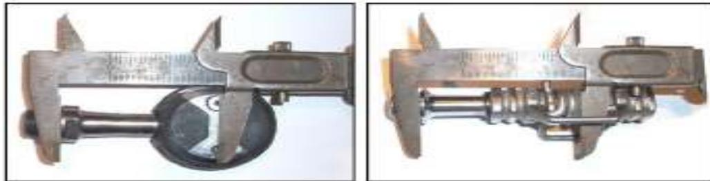
Figure 70. Pedal spindle length. Left: Speedplay X-1 titanium pedal top. 50 mm from crank face to center of pedal. Right: Crank Bros Egg Beater. 57 mm from crank face top center of pedal.
