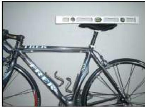
Figure 22. Saddle angle. The saddle is level.
