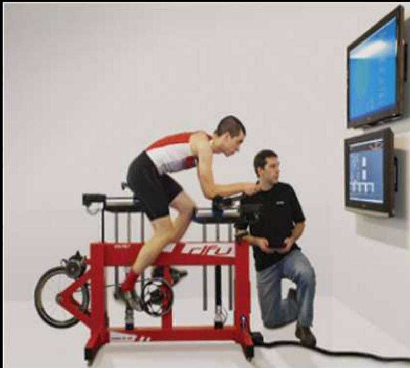
The DFU™, manipulates the rider's position while he or she is pedaling. The software, based on the client's body morphology, suggests a starting position for the fitter in using XY coordinates. The Guru trained fitter then adjusts the fit down to the millimetre in order to achieve a perfect fit, which is optimized for power, cadence, position and most of all, comfort
