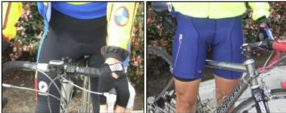
**Figure 2. Road bicycle frame size. Left: Allow at least 1 inch of clearance between the top tube and your crotch. Right: Compact road frames, like mountain bikes, will allow even more room.**
