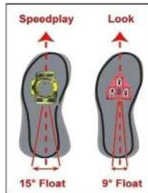
Figure 29. Both Speedplay (15°) and Look (9°) pedals have appreciable float.
