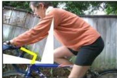
Figure 51. Computer generated image rotating around the shoulder. The torso angle is unchanged. Now the stem would be about 130 mm long with a 100-degree angle from the steering axis, about 4 inches above the headset. Although the torso angle is the same, the shoulder angle and handling characteristics of the bicycle have changed. This position is not recommended. See the text.
