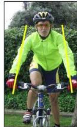
Figure 34. Mountain bike Pro and NORBA Champion Jimena Fiorit prefers the control that this wider-than-shoulder width handlebar provides.
