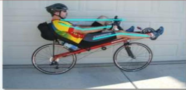
The reference model for fitting a Bacchetta high racer.
