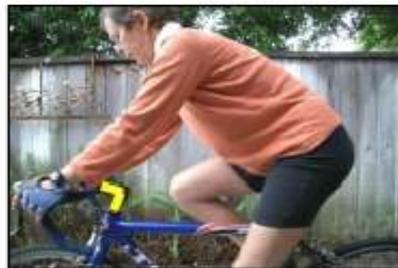
Figure 50. Yellow line marks a 60-mm long stem with a 90-degree angle from the steering axis, 2-1/4 inches above the headset.
